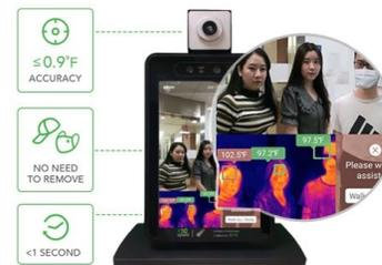
An infrared thermal camera and integrated display computer are calibrated to remotely measure the forehead and face surface temperatures. A 50-point scan, captured in under one second, is used to compute the 'core' body temperature to an accuracy of 0.3°F.
